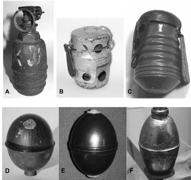
Figure 19. Five grenades and a lamp suspension egg. (A) A World War I American Mk II gas grenade. (B) A World War II Italian OTO 35 practice grenade. (C) An Italian Breda 35 “red devil” grenade. (D) This 1914 French OF1c ball grenade is almost identical to the French M61 grenade (not shown). (E) A lamp suspension egg. (F) A 1914 French suffocating gas grenade.
